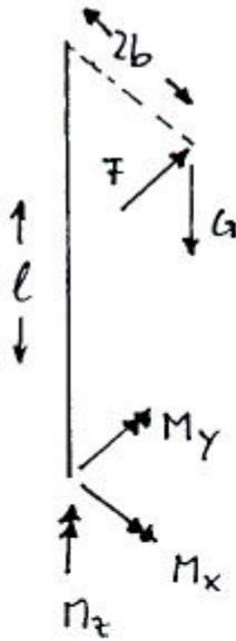
$$\left. \begin{aligned} M_x &= F \cdot l \\ M_y &= -2Gb \\ M_z &= -2Fb \end{aligned} \right\} \begin{array}{l} \text{Biegung} \\ \text{Torsion} \end{array}$$
